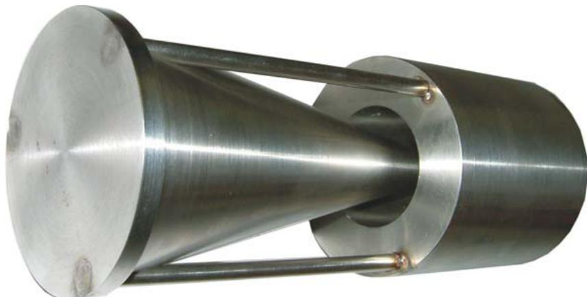
An effects head which is mounted above the area to be "fogged".
