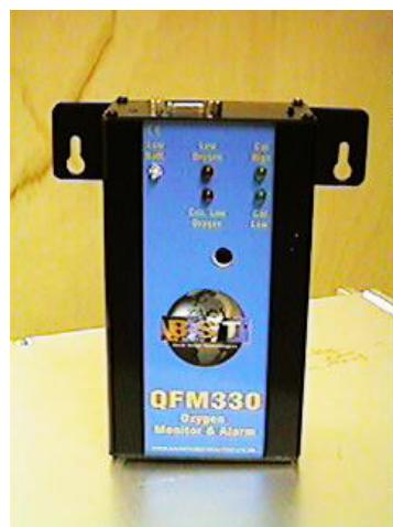
An oxygen depletion monitoring system is also included and integral to the controller. A remote sensor is mounted centrally in the club, this connects to the controller which then monitors the oxygen levels 24 hours a day and can not be switched off. Should oxygen levels drop to a level that could be deemed harmful then the controller will automatically shut down and lock-out. To re-enable the system a second key holder is required to reset the system.
