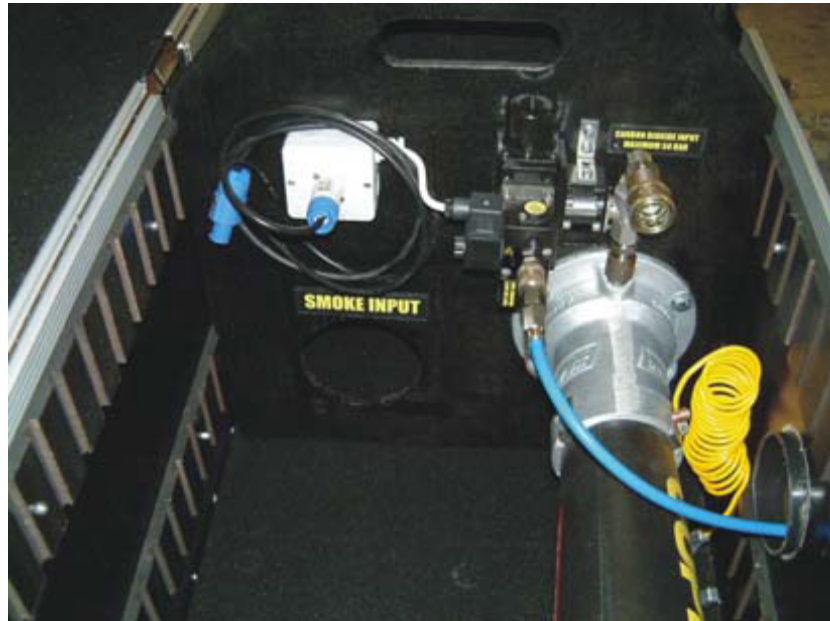
This shows the connection of the (blue) pneumatic hose and the power cable from the G300 smoke machine.
